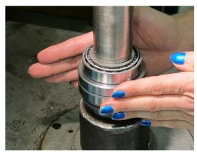
5. Press down the small tapered roller bearing in small steps until correct preload is achived. Not to tight and no backlash.
