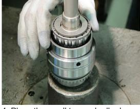
4. Place the small tapered roller bearing on the shaft as on the picture.
