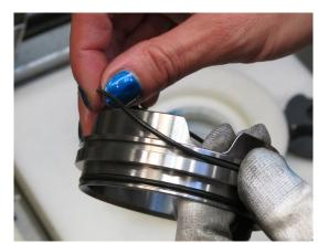
11. Assemble the O-rings on the distance ring.
