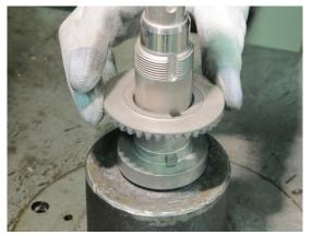
1. Place the ring gear on the shaft with the guide pin located against the guide hole.
