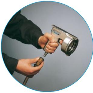
Connect the ***ptc*system®** launcher to the compressed air network or a compressed air cylinder.
