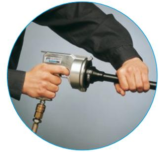
Close the ***ptc*system®** launcher and position the nozzle on the end of the tube or hose. Now press the trigger until the cleaning projectile is discharged from the end of the line.
