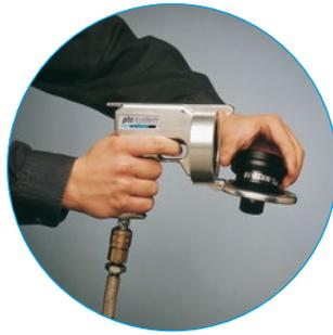
Select the appropriate nozzle and insert it into the open retaining ring on the ***ptc*system®** launcher. For assistance with the nozzle selection, see the operating manual and the tables starting on page 17.
