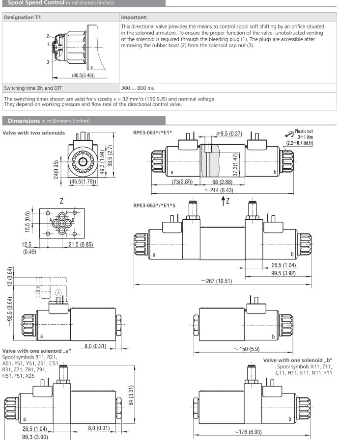
Mounting screws 🎣 8.9+1 Nm (6.56+0.7 lbf.ft) M5x45 DIN 912-10.9
