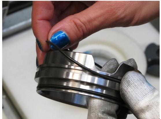
11. Assemble the O-rings on the distance ring.
