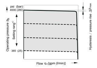
In order to prevent damage to the pump and the system, this setting range is the permissible setting range and must not be exceeded. The range of possible settings on the valve are wider.
