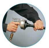
Close the **ptc**system<sup>®</sup> launcher and position the nozzle on the end of the tube or hose. Now press the trigger until the cleaning projectile is discharged from the end of the line.
