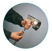
Connect the **ptc**system<sup>®</sup> launcher to the compressed air network or a compressed air cylinder.
