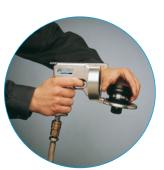
Select the appropriate nozzle and insert it into the open retaining ring on the **ptc**system<sup>®</sup> launcher. For assistance with the nozzle selection, see the operating manual and the tables starting on page 17.
