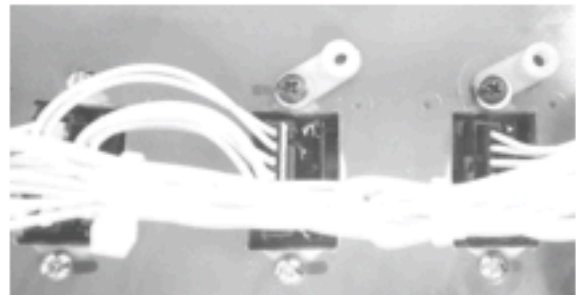
New joystick with new PCB mountings: thread rolling screws, washers and M3 insert feet
