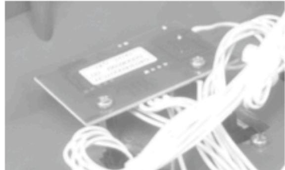
Present PCB assembly with mountings (zinc plated M3 screws and threaded metal spacers)
