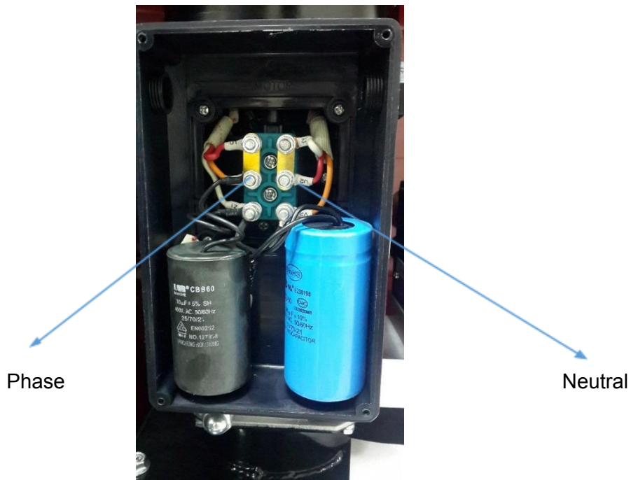
Photo 5. Connection on 220 V AC mono phase motors*
