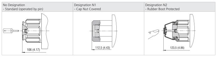
In case of solenoid malfunction or power failure, the spool of the valve can be shifted by manual override as long as the pressure in port T does not exceed 25 bar (363 PSI). For alternative manual overrides contact our technical support.
