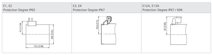
The indicated IP protection level is only achieved if the connector is properly mounted.
