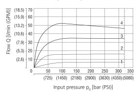
Nominal flow 60 l/min (15.85 GPM)
