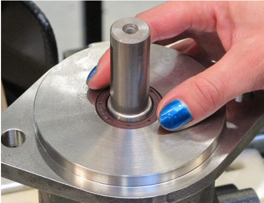
19. Carefully push down the shaft seal.
