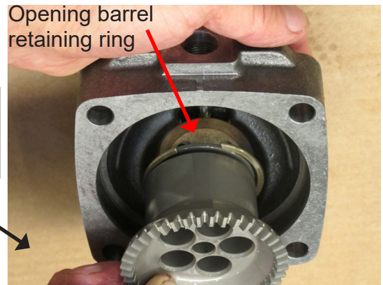
5. Assemble the cylinder barrel as shown in picture.
